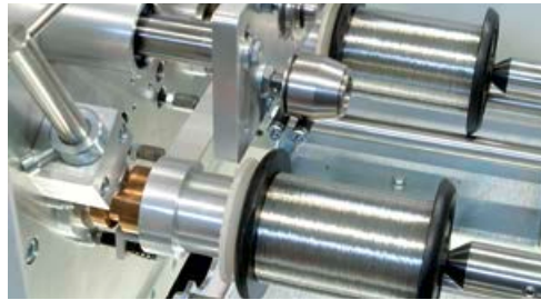
DSH-L: semi-automatic wire winding machine with 2 spindles
