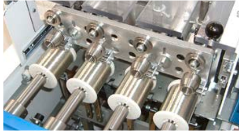
DSA-L: automatic wire winding machine with 4 and 2 spindles
